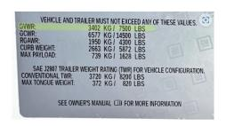
WARNING: Use the weight in pounds from this mylar sticker. DO NOT use the registered weight from the registration certificate. If the sticker is missing from inside the door, use VIN Assist link to check for the vehicle's minimum GVWR".
